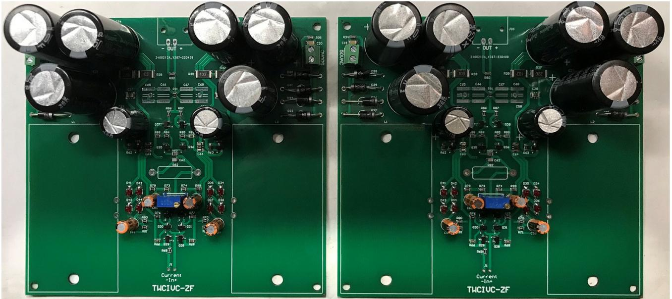
TWCIVC-ZF DAC current to voltage converter without global feedback and inductive power supply.
