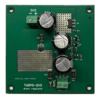
Low noise voltage shunt regulator designed to provide power supply to the isolated side of the TWSAFB-XMOS and the TWSAFB-USB I2S/DSD over USB interface.
