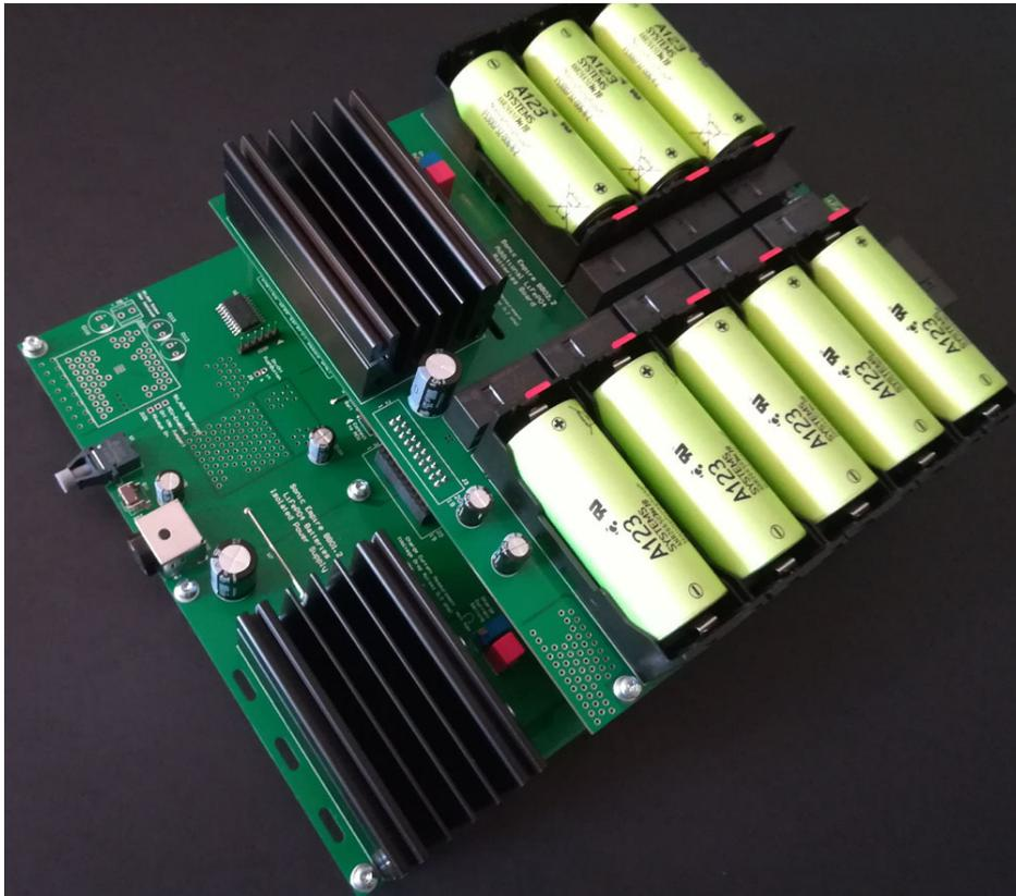
This board is part of the new LiFePo4 batteries power supply system. This is an extra board intended to add more rails to the main board. It's controlled by the main board processor.
