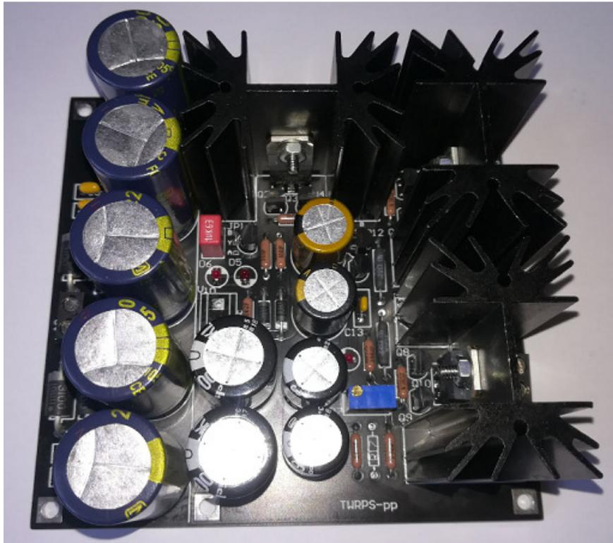
Low noise linear push-pull regulator designed to provide power supply to the oscillators and the frequency doublers.
