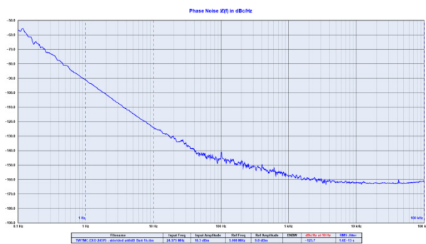
TWTMC-EXO 24.576 MHz phase noise
