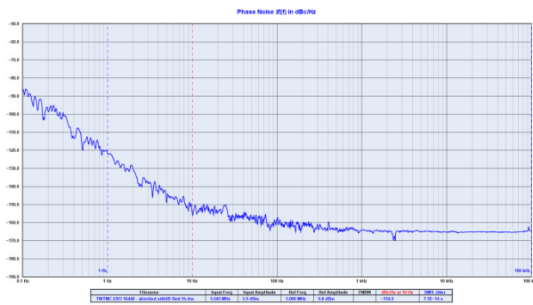
TWTMC-EXO 5.6448 MHz phase noise
